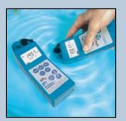
The 6Pfc measures a dynamic range of free chlorine concentrations wider than the range of colorimetric test kits.
